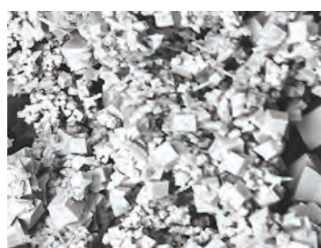
Microscopic view (x5000) of well developed copper hydroxide {Cu(OH) 2 } protective layer formed on the inner surface of TALOS copper tube.
